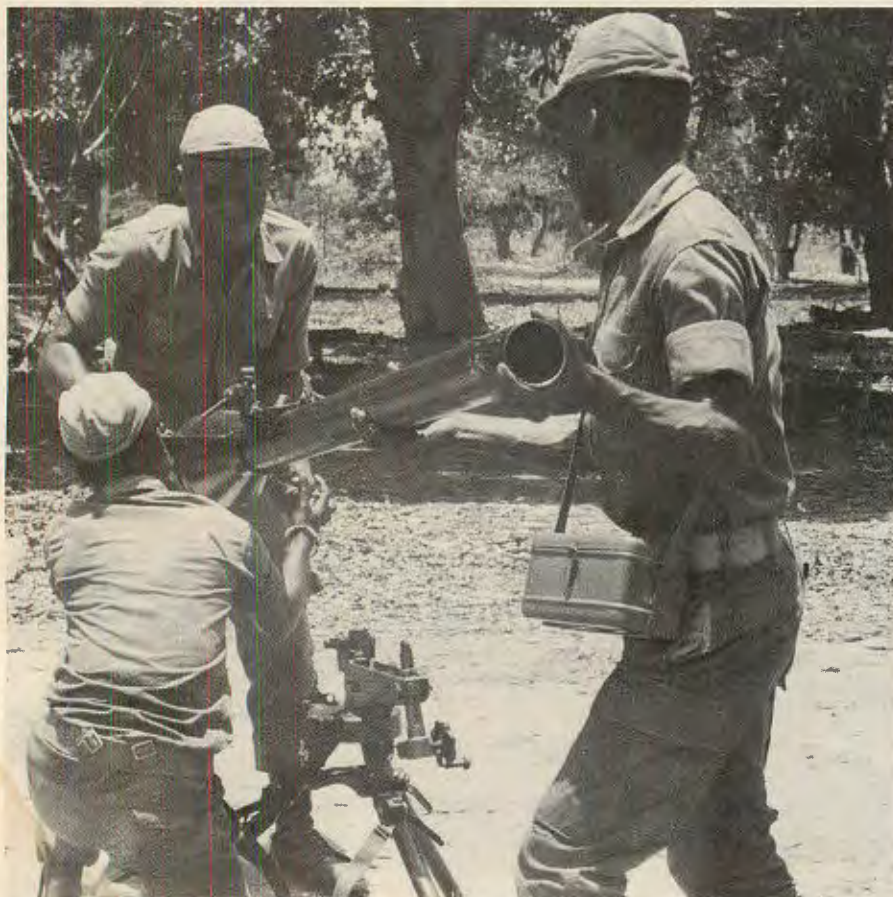
LEFT: UNITA forces in Eastern Angola assembling captured Type 52 Chinese-built 75mm recoilless rifle, direct copy of U.S. M20. Container carried by soldier in foreground contains weapon's sights. BELOW: Large numbers of Soviet war supplies are being captured on regular basis from SWAPO bands. RIGHT: Russian-supplied MPLA forces with AK-47s during flag-raising ceremony north of Luanda.
